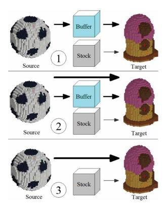
**Figure 4.** Three strategies under each approach. Strategy 1: Disassemble the source model completely to a buffer; then build the target from the buffer and a stock. Strategy 2: Build the target from the source, a buffer (disassembled bricks from the source), and a stock. Strategy 3: Build the target from the source and a stock. The size of arrow represents its priority to move.
