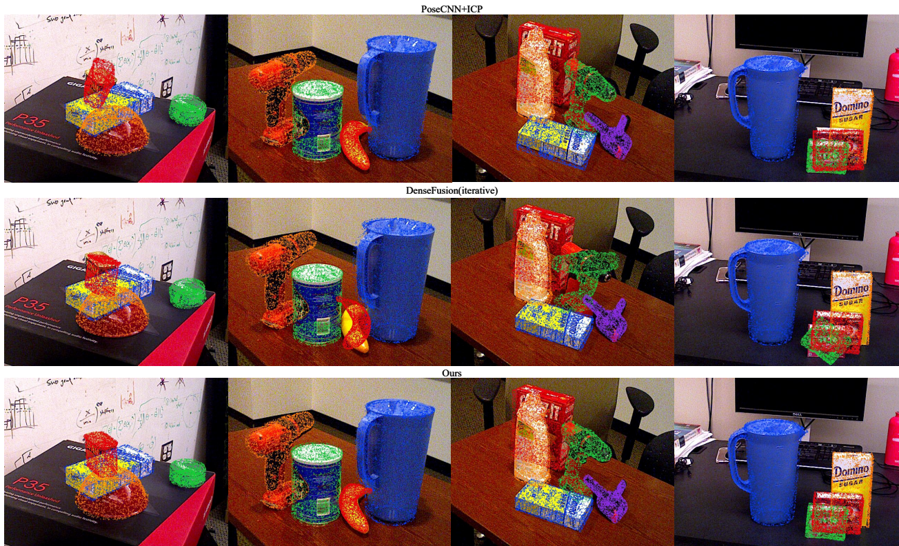
Figure 8: Visual comparison of estimated poses. Various colors and shapes represent the same object visualized as point clouds using different methods.
