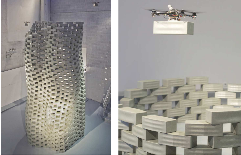
FIGURE 1.5: The Flight Assembly System (Augugliaro et al., 2014). (a) The Flight Assembled architecture installation. The 6-m-tall tower consisting of 1500 foam elements was assembled by four quadcopters in France, 2011. (Photograph by François Lauginie.) (b) Placing a module. The vehicle hovers above the structure before placing a construction module.
