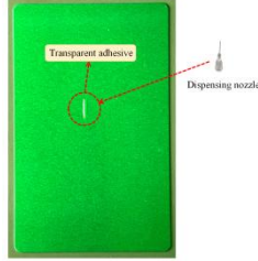
Fig. 1. Schematic of designed transparent adhesives specimen.
