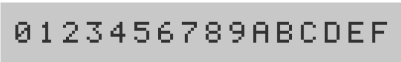
Figure 28.1: Training row of the custom dot-matrix font: 16 characters, 0–9 and A–F, each 20×28 px, ink gray 50 on background 200. The character set deliberately includes confusable pairs such as 0/D and 8/B, planting the seed for the confusion experiments to come.
