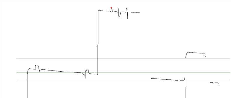
Figure 42.3: Height profile along the vertical center line x = 16.1 mm (black curve). From left to right it passes through the upper plateau, the central boss top (peak 5.987 mm, red dot), the step, the lower plateau, and the low boss; the two horizontal lines are the upper/lower plateau references. The two downward notches on the boss top are the top-face pits.
