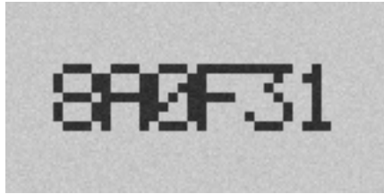
Figure 28.4: Test string with character spacing squeezed to 0: the strokes of the first 5 characters “8A0F3” touch and merge into a single connected component, and only the ‘1’ stays separate. The segmenter extracts 2 “characters”, and the recognition result is “?1”.
