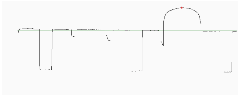
Figure 41.4: The x - z cross-section at the row through the bump peak: the black polyline is the real height along that row, the green horizontal line marks the land datum and the brown line the channel-floor datum; the polyline dropping 4.4 mm back and forth between them is the step, and the dome rising above the green line with a red dot at its apex is the bump defect (2.518 mm above the land).
