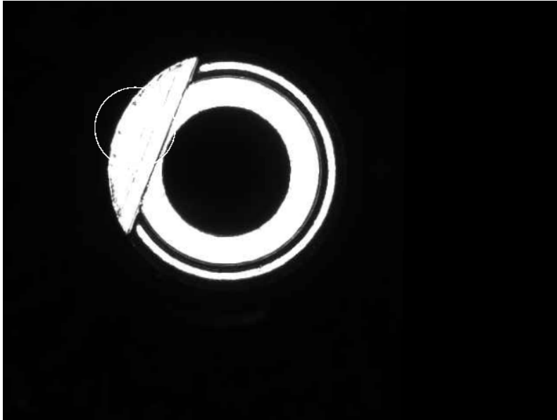
Figure 19.3: After the current image (002) is rotated back to the reference pose by the fixturing matrix, the original ROI measures. The part returns to 001's layout, and the original ROI again covers the tab.
