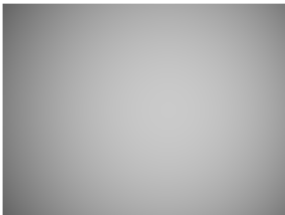
Figure 4.3: Flat-field reference image: imaging a uniform white board, the resulting brightness distribution is the pure gain field of the illumination system — dark on the left and bright on the right, dark in the corners and bright in the center, exactly the same structure as Figure 4.1b.
