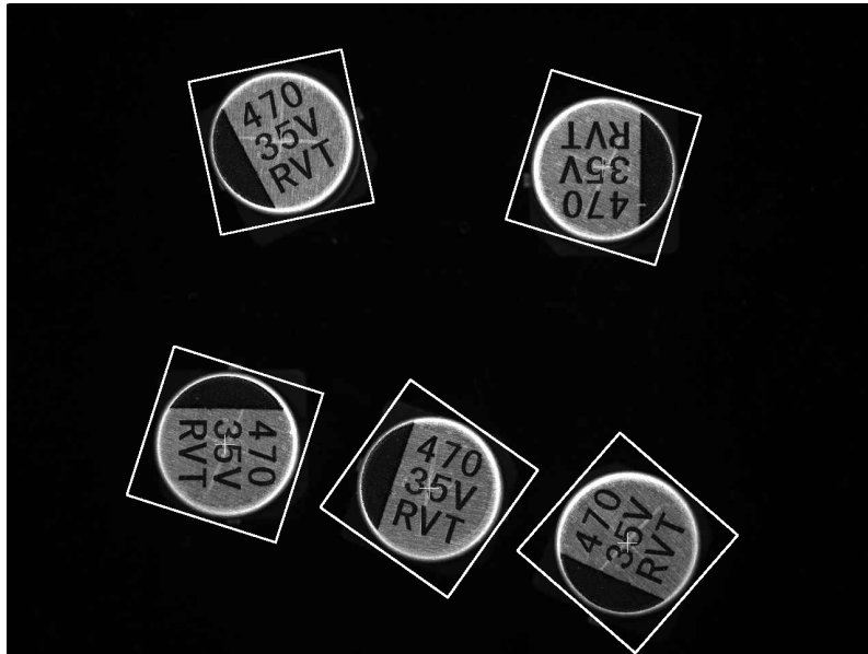
Figure 16.3: The search results of FindGreyImageModel on sample 003: all five capacitors found — crosses mark the subpixel centers, white boxes mark the matched poses — including the nearly 180^\circ flipped instance and the large-angle rotated ones; none is falsely detected on the black background.
