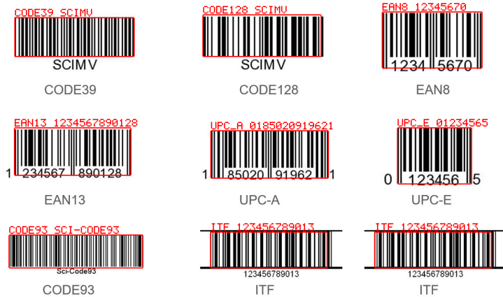
Figure 27.1: Real multi-symbology 1D barcode test card sample/barcodes.jpg (1536×878 grayscale): a standard card carrying 8 symbologies / 9 symbols — top row: CODE39 and CODE128 both encoding “SCIMV”, EAN-8 encoding 12345670; middle row: EAN-13 encoding 1234567890128, UPC-A encoding 185020919621, UPC-E encoding 01234565; bottom row: CODE93 encoding “Sci-Code93”, two ITF (Interleaved 2 of 5) both encoding 123456789013. The red boxes and red labels are SciVision FindBarcode detections overlaid (symbology name + decoded string).
