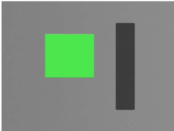
Figure 38.6: Height threshold segmentation result: the boss separated by height > 1200 m is highlighted in green overlaid on the gray-value height base map. Segmentation 7197 pixels vs. ground truth 7200, FP = 0, FN = 3, IoU = 0.9996.
