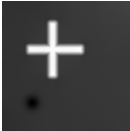
Figure 34.5: Height map obtained from the normal field by Poisson (SOR) integration. The slowly varying dent is recovered well, the logo’s steep wall has its height underestimated due to self-shadowing, and a slight low-frequency drift exists at the four corners.
