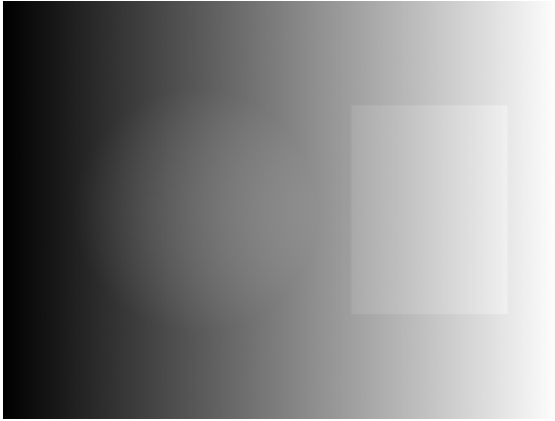
Figure 32.4: Absolute phase after dual-frequency hierarchical unwrapping. All wrapping cliffs are smoothed out, the phase rises continuously and monotonically with height, and the spherical cap (the central dome) and the step (the block on the right) are obvious at a glance.
