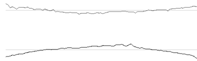
Figure 21.4: Straightness deviation profile (normal deviations \times 40 , horizontal axis is position along the edge): top, the left long edge (0.624 px, fairly straight); bottom, the right long edge (0.872 px, with a gentle bow and a local bump).
