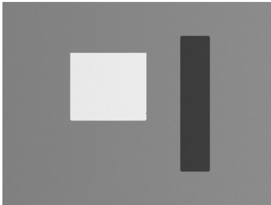
Figure 38.4: Range image after morphological closing for hole filling: the originally scattered black invalid pixels (3858 of them) are almost all filled with the median of valid neighbors (1 remaining), and the surface regains continuity.
