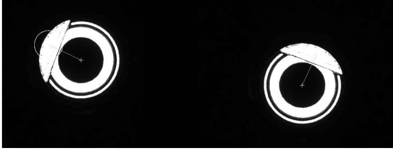
(a) Reference scene (sample 001): the ring center (cross) plus the direction line to the tab; the inspection ROI (white circle) sits on the tab (b) Current scene (sample 002): the same part translated by (+78.9, +81.0) px and rotated by about 90°; the white cross is the located ring center
